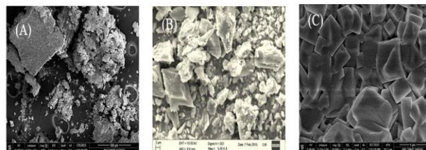
Figure 4 SEM Images of (A) (\text{NH}_4)_3(\text{PW}_{12}\text{O}_{40}) (B) [CuComplex] (C) (\text{NH}_4)_3[(\text{CuComplex})(\text{PW}_{12}\text{O}_{40})]
